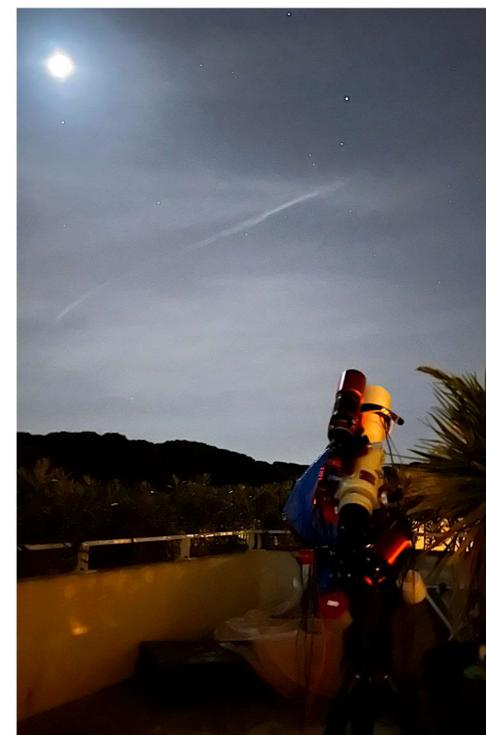
Setup: Takahashi FSQ85ED refractor (D=85mm F/5). Star'Ex LR spectrograph (15 microns slit). Main camera ZWO ASI533MM pro. Mount ZWO AM5. Guiding by using ASIair system. Prism software for spectra acquisition. Star'Ex project: <http://www.astrosurf.com/solex/>
